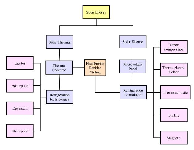
**Figure 1.** Classification of solar refrigeration systems (Kim and Ferreira, 2008; Papadopoulos et al., 2003; Ewert et al., 1998).
