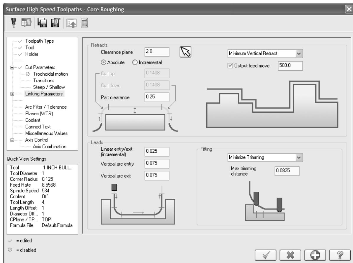
**Linking** options allow you to configure how Mastercam links air moves when the tool is not in contact with the part
