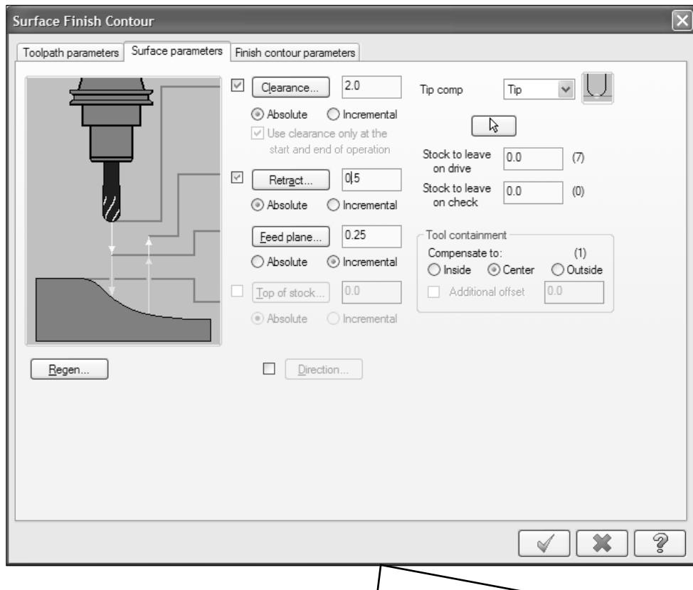
**Clearance** value sets the height at which the tool rapidts to or from the part.
