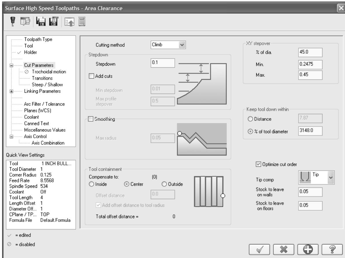
**Step-down** options allow you to configure how Mastercam spaces the cuts in Z.
