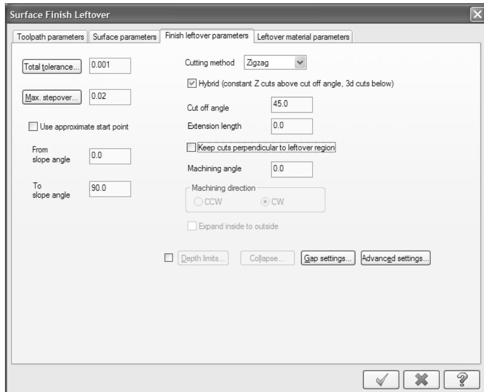
**Total tolerance** is the sum of the filter tolerance and cut tolerance. You can adjust the ratio of the filter tolerance to the cut tolerance, change the tolerance amounts, and select arc options.
