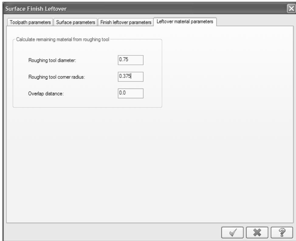
**Roughing tool diameter** is the diameter of the previous tool that was used to machine the part (in our case the 0.75 " Ball endmill used in the finish contour toolpath).
