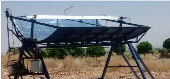
Fig. 2. Reflection of the sun's rays on the pipe at the focal point of the parabolic collector.
