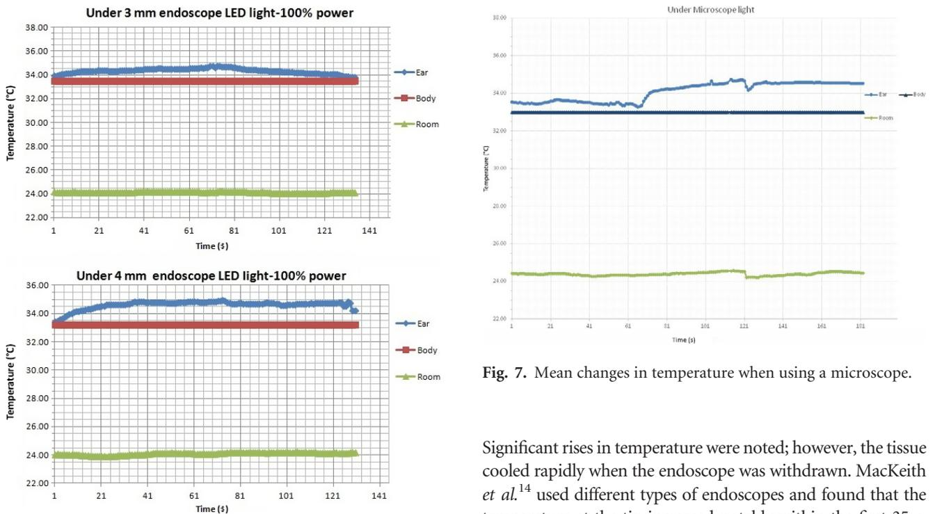
Fig. 6. Mean changes in temperature when using a 3- or 4-mm-diameter rigid endoscope with light-emitting diode light sources.
