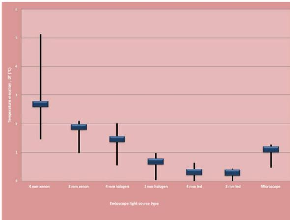
Fig. 8. Minimum, maximum and average increases in temperature when using different light sources.
