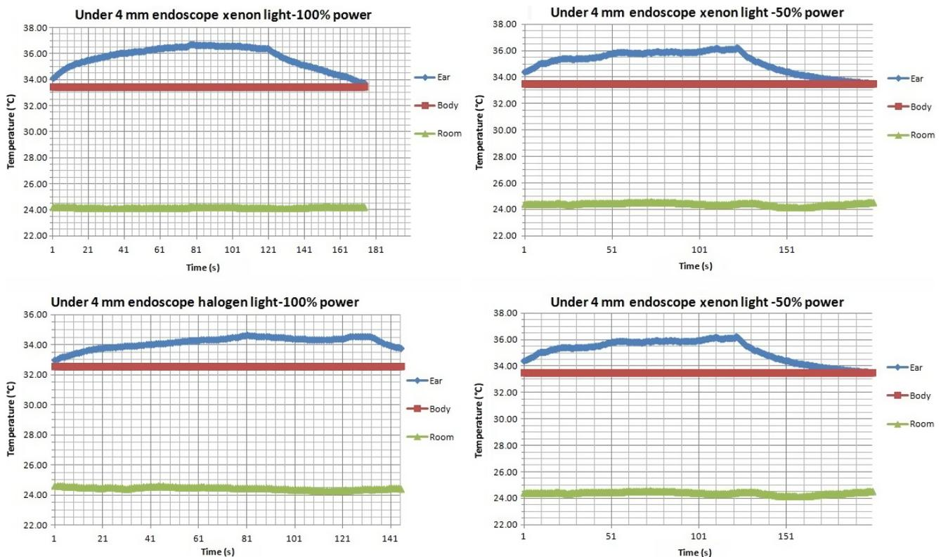
Fig. 4. Mean changes in temperature when using a 4-mm-diameter rigid endoscope with halogen and xenon light sources.
