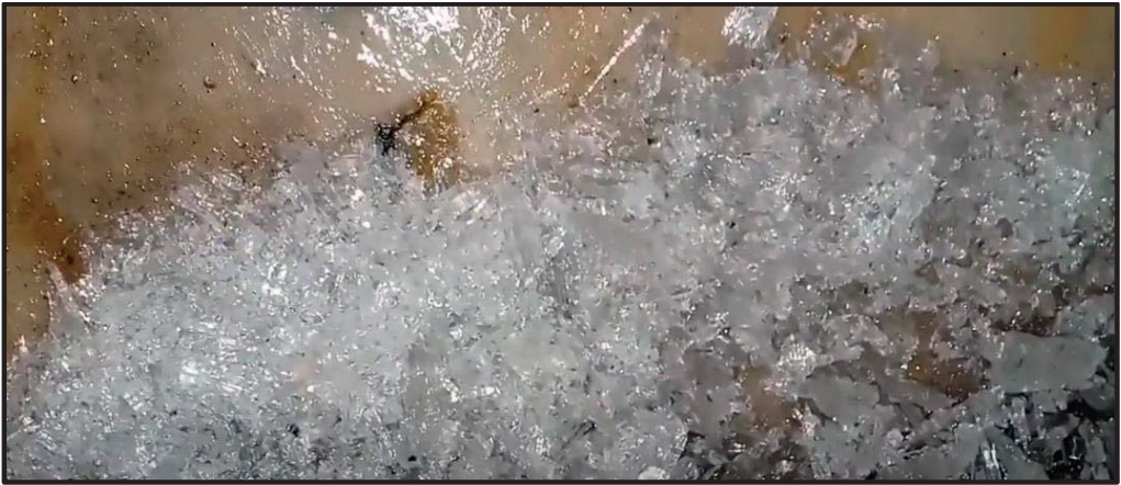
Figure 3. Crystallization of LiBr/Water solution
