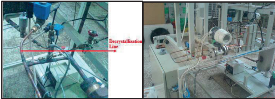
Figure 8. Decrystallization line of the experimental set-up
