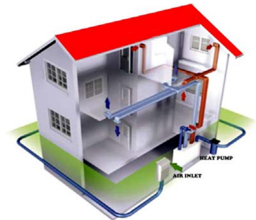
Figure 4. EAHX integrated with mechanical ventilation or heat pump. [7]
