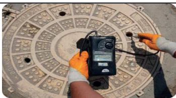
Figure 4. Manhole Cover Leakage Test
