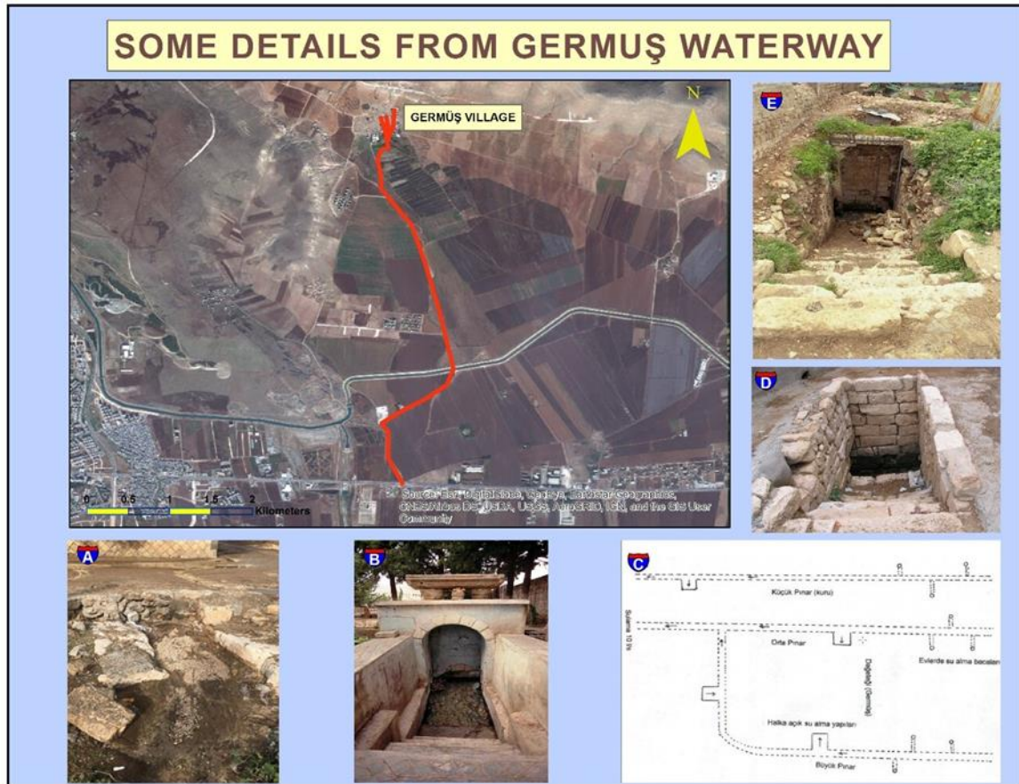
Figure 5. The route of the Germüş Water and its details. a) The middle and big springs were connected and continued in an open channel. b) A kehriz water is using in structures, made of regularly cut stone and were taken down by stairs in houses, (Uceymi Sadun Pasha House), c) The plan of kehriz system of Germüş (from Bildirici, 2009), d) A water usage structure on a kehriz system in the village square. It is also a ventilation structure. e) An another ventilation and water usage structure on dry kehriz spring.
