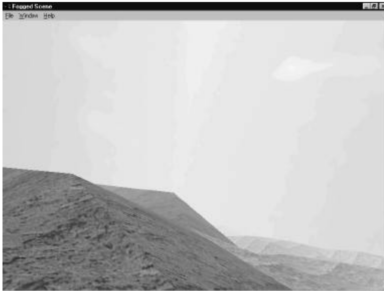
Figure 16-5 Weather haze using glFog
