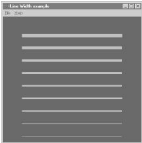
Figure 6-9 Demonstration of glLineWidth from LINESW program
