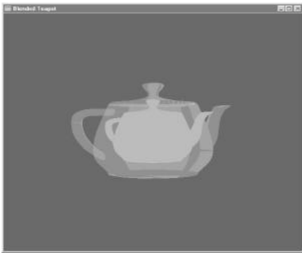
Figure 16-1 Transparent teapot using blending
