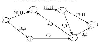
$\begin{array}{c} \textbf{Remove all the labels. Start scanning} \\ \text{If we try paths} \\ 1,2,5,3,6 \\ \text{we will get} \quad \Delta_t = 0 \\ \textbf{Result: We have reached maximum flow.} \end{array}$
