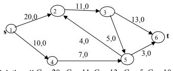
Solution 1)  $C_{12}=20$ ,  $C_{23}=11$ ,  $C_{36}=13$ ,  $C_{35}=5$ ,  $C_{14}=10$ ,  $C_{45}=7$ ,  $C_{52}=4$ ,  $C_{56}=3$ ,  $f_{12}=f_{23}=f_{36}=f_{35}=f_{14}=f_{45}=f_{52}=f_{56}=0$ ,
