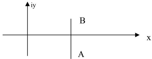
The straight line from A=1-i to B=1+3i is a parallel line to the y axis. x is constant(x=1). thus  $dx=0$ .
