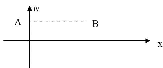
The straight line from A=i to B=i+2 is a parallel line to the x axis. y is constant(y=1). thus  $dy=0$ .
