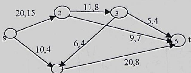
First number: capacity ( $C_{i,j}$ )Second Number: given flow ( $f_{i,j}$ )
