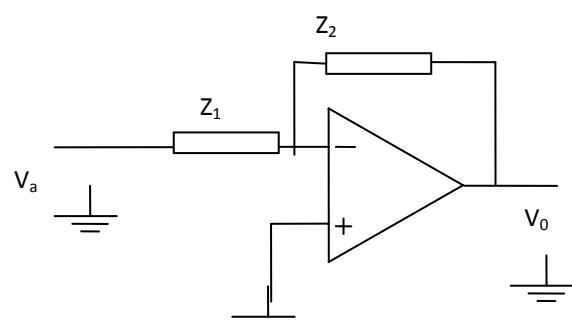
1) 562) Find the transfer function  $\frac{V_o(s)}{V_i(s)}$  of the following circuit.
