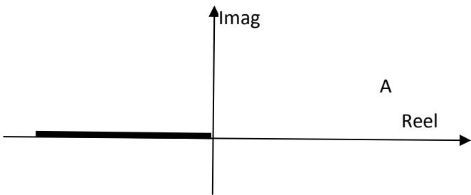
$$\begin{aligned} Y &= KG(X-Y) \\ Y+KGY &= KGX \\ Y/X &= KG/(1+KG) \end{aligned}$$
