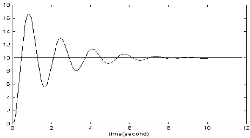
6) The input to the following system is  $r(t) = 10u(t)$  ( $u(t)$  is step function). The output are given below. Calculate approximate value of  $e_{ss}$  steady state error.
