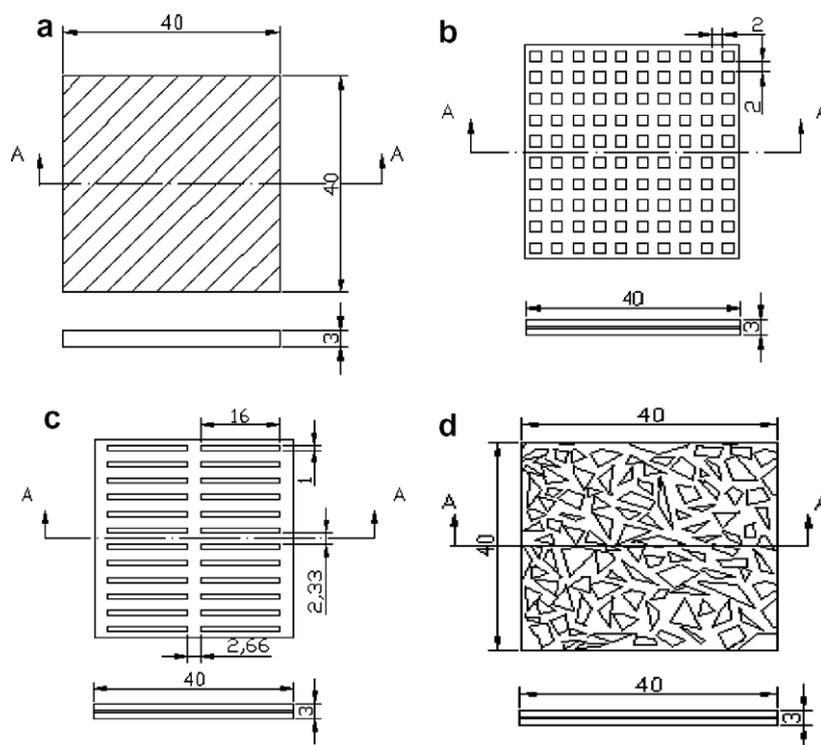
Fig. 1. Geometric specifications of the specimens; (a) ordinary concrete, (b) concrete with strip PET pieces, (c) concrete with square PET pieces, (d) concrete with irregular PET pieces.
