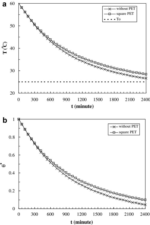
**Fig. 3.** The transient temperatures for specimens of ordinary concrete and concrete with square PET pieces: (a) in dimensional form and (b) in dimensionless form.
