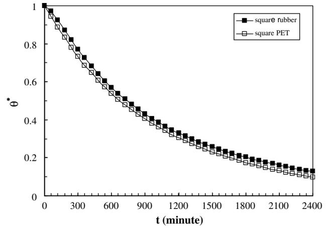
**Fig. 5.** Dimensionless transient temperatures for specimens of concretes with PET and rubber pieces of square shapes.
