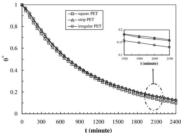
**Fig. 4.** Dimensionless transient temperatures for specimens of concretes with PET pieces of various shapes.
