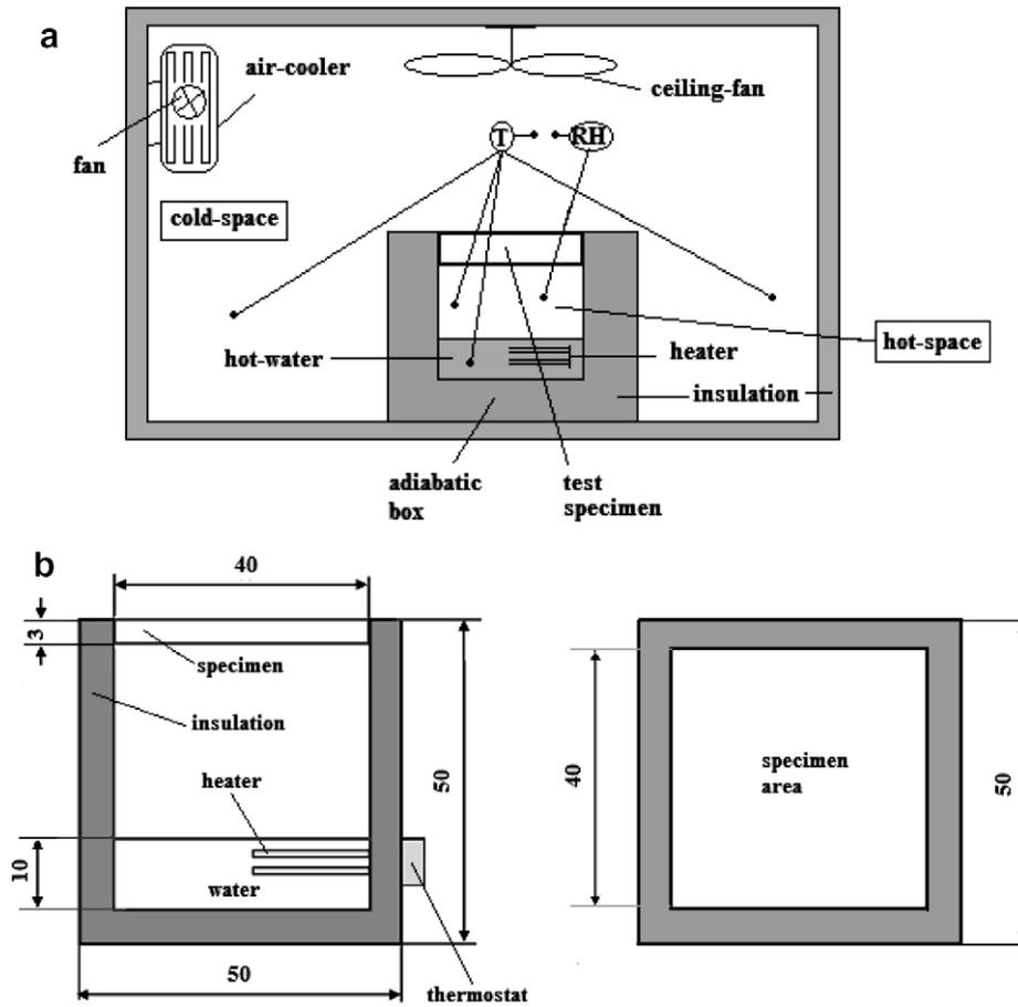
Fig. 2. (a) Schematic of the dynamic adiabatic-box apparatus (T: temperature sensor, RH: relative humidity sensor) and (b) dimensions of the adiabatic-box (in cm).
