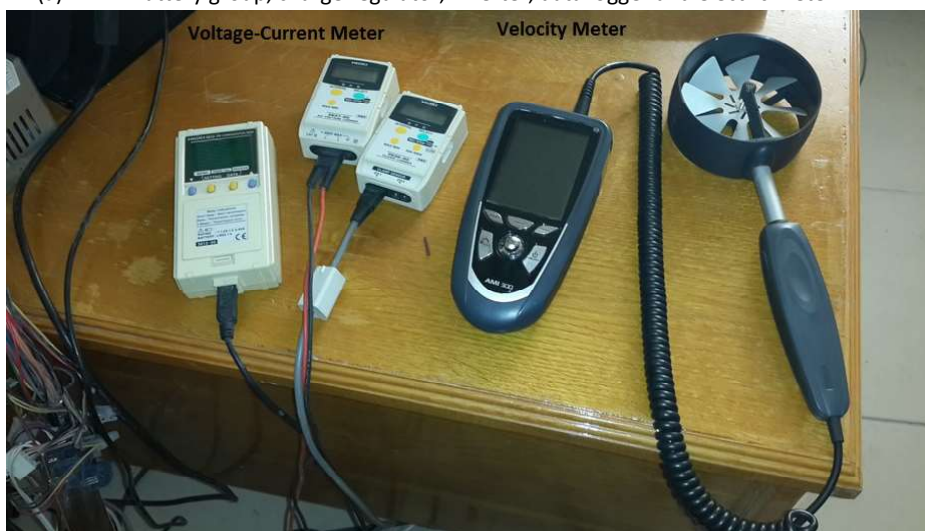
(a) Voltage-current meter and velocity meter
