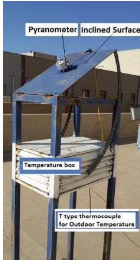
Figure 4. Solar radiation measurement by a pyranometer.
