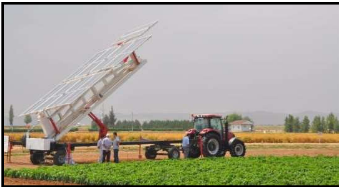
Figure 1. Mobile solar powered irrigation system.
