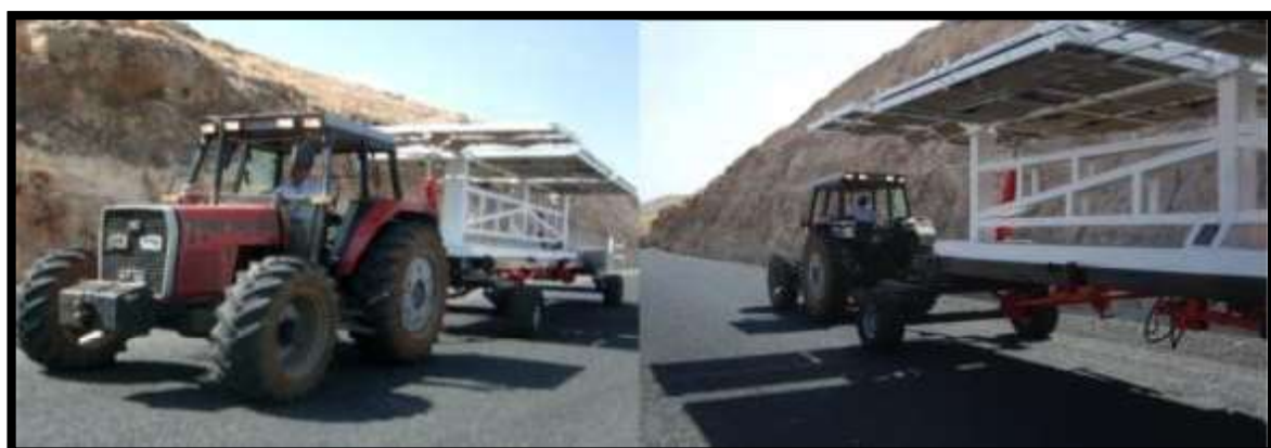
Figure 2. The transportation of the mobile solar irrigation system
